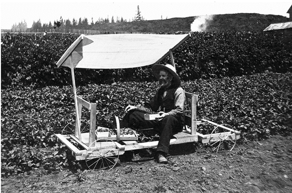
Edward Abbott picking strawberries on his farm using his invention—a wheeled platform with a canopy offering protection from the hot sun which one could lie on and push between the rows with your feet. It had a slotted centre from which to pick berries and space for placing the fruit baskets.
